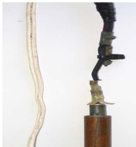
Figure 10.2 Close-up of the probe at the end of the cable showing the upper bared end and the lower end soldered to the metal weight.
