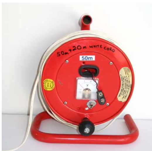
Figure 10.1 Hand-winch and twin-core cable set-up, fitted with a voltmeter for water level measurement. The 6 volt battery fitting for the voltmeter is dangling next to the voltmeter
